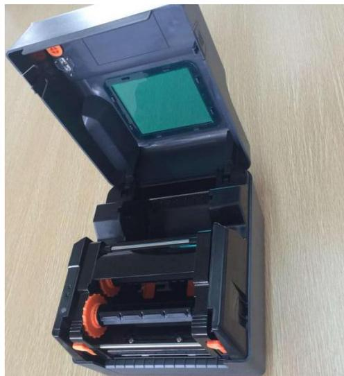
3. Make the left side of recovery shaft (Hexagonal side) pressed into the ribbon recovery wheel,
