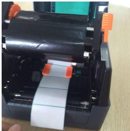
6. With both hands press down as the left arrow's photo, close the print head. Please make sure that the print head is completely closed, to ensure the printing quality.
