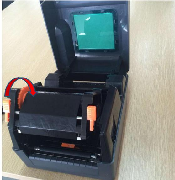
8. According to the direction of the arrow rotating ribbon recovery wheel, until the ribbon black areas cover the printing head and tightly ribbon, to make no any folds of the ribbon
